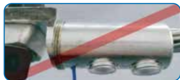
High bolt protrusion
